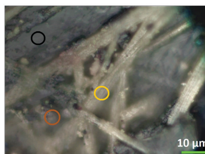
Fig. 2 (a) Raman spectra of the polymorphism of a degraded \text{FAPbI}_3 SC associated by color with the measurement point shown in (b) the microscope image (magnification \times 10 ).
