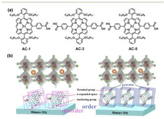
**Fig. 10** (a) Chemical structures of AC-1, AC-3, and AC-5. (b) Schematic diagram of interfacial changes between ITO/SAM/perovskite. Reproduced with permission.<sup>74</sup> Copyright 2023 Wiley-VCH GmbH.
