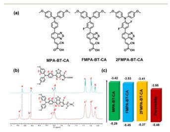
**Fig. 12** (a) Molecular structures of MPA-BT-CA, FMPA-BT-CA, and 2FMPA-BT-CA. (b) Comparison of the <sup>1</sup>H NMR spectra of MPA-BT-CA with or without Pbl<sub>2</sub>. Reproduced with permission.<sup>77</sup> Copyright 2023 American Chemical Society. (c) Diagram of the device energy level alignment. Reproduced with permission.<sup>80</sup> Copyright 2023 American Chemical Society.
