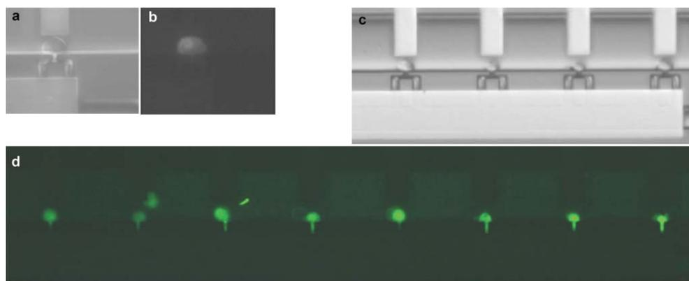
**Fig. 2** Electroporation and transport PI and expression of EGFP-N1 into C2C12 cells. Proof of principle; (a) bright field and (b) fluorescence image of C2C12 cell showing PI uptake after a pulse of 2 V and 6 ms; (c) immobilised C2C12 cells in the microfluidic device before electroporation; (d) Overview of all nine cell traps in the chip: electroporation of EGFP-N1 in C2C12 cells resulted in 100% transfection efficiency after 24 h, as visible by EGFP expression.
