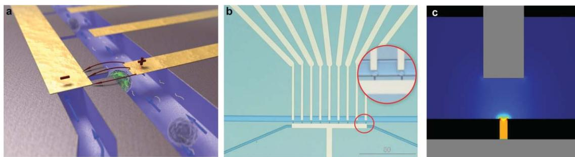
**Fig. 1** Silicon-glass microfluidic device for single cell electroporation and gene transfection studies (20  $\times$  15  $\times$  1 mm) (a) Artistic 3D impression of trapped cells; (b) Microfluidic chip layout, zoom-in on trapped single cells; (c) Analysis of the electric field strength distribution at the trapping sites shows that a voltage of 1 V yields an electric field strength of 0.57  $\text{kV cm}^{-1}$ .
