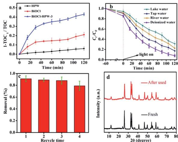
Fig. 6 TOC removal of TC in the presence of BiOCl, HPW and BiOCl-HPW-3 within 120 min illumination (a), removal of TC in the presence of BiOCl-HPW-3 in real wastewater (b), the recyclability test (c) and XRD patterns (d) of BiOCl-HPW-3 (photocatalyst concentration was  $0.2 \text{ mg mL}^{-1}$  and TC concentration was  $10 \text{ mg L}^{-1}$ ).
