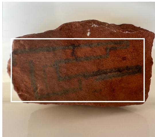
Fig. 1 Top view of a Bauxite sample as an example of a mineral used in LIBS analysis. The white rectangular box marks the area where the laser spots were applied during measurements.
