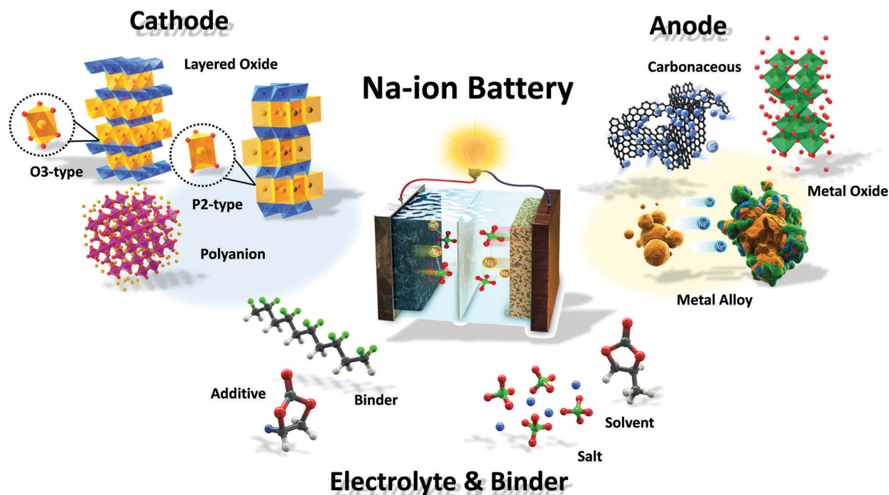
Scheme 1 Illustration of a Na-ion battery system.
