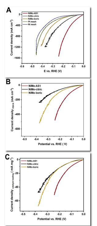
Fig. 1 (A) Linear sweep voltammetry (LSV) data showing geometric current densities of NiMo-AS1, NoMo-citric, NiMo-boric on Ni mesh support, bare Ni mesh, and Pt mesh; (B) LSV data showing electrochemical active surface area (ESCA) averaged current densities of NiMo- AS1, NiMo-citric, NiMo-boric deposited on Ni mesh: (C) LSV data showing catalyst loading averaged current densities of NiMo-AS1, NiMo-citric, NiMo-boric on Ni mesh
