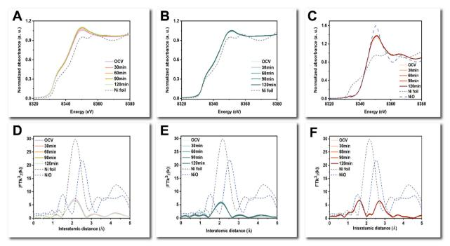
Fig. 6 Operando XAS data: (A)–(C)-Ni K-edge XANES spectra of A-NiMo-AS1; B-NiMo-citric; C-NiMo-boric; (D)–(F)-Ni K-edge  $k^3$ -weighted EXAFS spectra for D-NiMo-AS1; E-NiMo-citric; F-NiMo-boric during activation in 1.0 M KOH.
