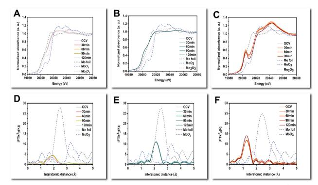
Fig. 7 Operando XAS data: (A)–(C)–Mo K-edge XANES spectra of A-NiMo-AS1; B-NiMo-citric; C-NiMo-boric; (D)–(F)–Mo K-edge  $k^3$ -weighted EXAFS spectra for D-NiMo- AS1; E-NiMo-citric; F-NiMo-boric during activation in 1.0 M KOH.
