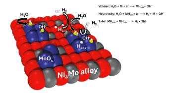
Fig. 10 Schematic diagram of synergetic catalysis of alloy-oxide interface structures, in which the molybdenum oxide promotes water dissociation, and the alloy accelerates hydrogen combination.
