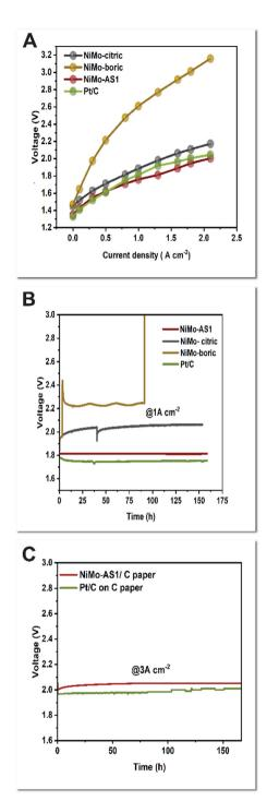
Fig. 3 (A) Polarization curves of AEMWEs with NiMo-AS1, NiMo-citric, and NiMo-boric on C paper as the cathode, respectively; (B) long-term electrolysis data at a constant current density of 1 A cm $^{-2}$  and cell temperature of 80  $^{\circ}$ C; (C) electrolysis at a current density of 3 A cm<sup>-2</sup> at 80 °C.
