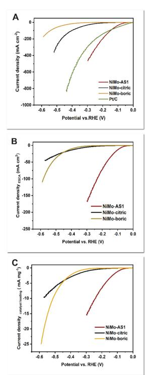
Fig. 2 (A) Linear sweep voltammetry data showing the geometric current densities of NiMo-AS1, NiMo-citric, NiMo-boric on C paper support and Pt/C sprayed on C paper support; (B) LSV data showing electrochemical active surface area (ESCA) averaged current density of NiMo-AS1, NiMocitric, NiMo-boric deposited on C paper support; (C) LSV data showing catalyst loading averaged current densities of NiMo-AS1, NiMo-citric, and NiMo-boric on C paper support.
