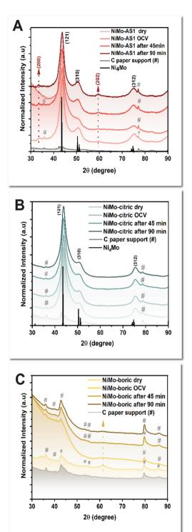
Fig. 5 (A) Operando XRD pattern of NiMo-AS1. (B) Operando XRD pattern of NiMo-citric. (C) Operando XRD pattern of NiMo-boric.
