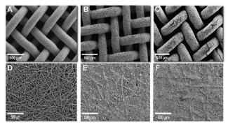
Fig. 4 (A) SEM image of bare Ni mesh; (B) SEM image of the as-prepared NiMo-AS1 on Ni mesh; (C) SEM image of the NiMo-AS1 on Ni mesh after HER at 1 A cm<sup>-2</sup>; (D) SEM image of the bare C paper; (E) SEM image of the as-prepared NiMo-AS1 on C paper; (F) SEM image of the NiMo-AS1 on C paper after HER at 1 A cm<sup>-2</sup>
