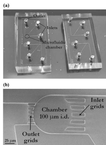
**Fig. 2** PDMS-based microfluidic systems used for confined sonoporation experiments on suspension cells. (a) Photograph of such a microsystems having dimensions of 1.8 cm  $\times$  0.8 cm (one system includes two independent devices); (b) SEM photograph of a 100  $\mu\text{m}$  diameter microchamber where cells are collected, scale bar denotes 25  $\mu\text{m}$ .
