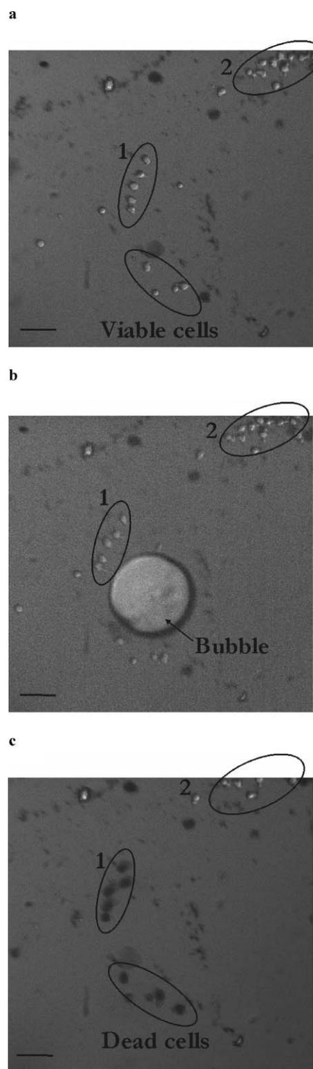
**Fig. 5** Determination of the interaction distance of a cavitation bubble with HL60 cells. Pictures of the microfluidic chamber (diameter 600  $\mu\text{m}$ ; height 35  $\mu\text{m}$ ) loaded with HL60 cells before (a), during (b) and 47 s after (c) exposure to a cavitation bubble. Black cells in (c) (group 1) have been affected by the cavitation bubble and are positive to trypan blue, whereas cells in group 2 remain viable. Scale bar denotes 50  $\mu\text{m}$ .
