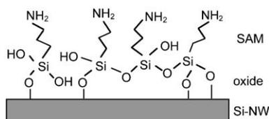
**Fig. 3** 3-Aminopropyltriethoxysilane (APTES) self-assembled monolayer on oxidized Si-surfaces with amine  $\text{NH}_2$  and hydroxyl  $\text{OH}$  terminal groups. Reprinted with permission from ref. 20 (*Langmuir*, 2000, **16**, 2651–2657). Copyright 2000 American Chemical Society.
