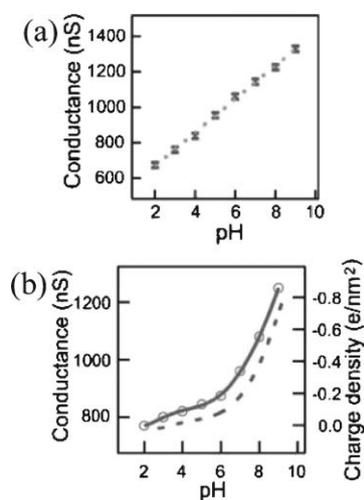
**Fig. 4** Si-NW conductance *versus* pH for (a) modified oxide surfaces and (b) unmodified oxide surfaces. (a) Reprinted with permission from ref. 4 (*Science*, 2001, **293**, 1289–1291). Copyright 2001 AAAS. (b) Reprinted with permission from ref. 51 (*J. Phys. Chem.*, 1957, **61**, 1166–1169). Copyright 1957 American Chemical Society.
