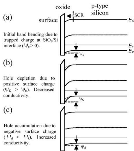
**Fig. 2** Qualitative band-bending diagrams for oxidized p-type Si-NW surfaces. (a) Initial band bending due to  $\text{SiO}_2/\text{Si}$  charge resulting in hole depletion, (b) negative surface charge at oxide surface resulting in increased hole depletion (decreased conductance), (c) positive surface charges leads to hole accumulation (increased conductance).
