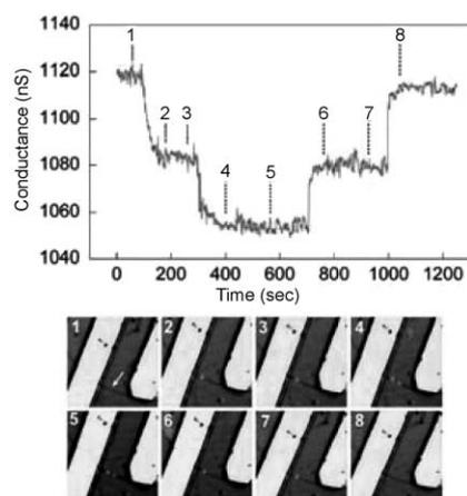
**Fig. 8** Simultaneous conductance and optical *versus* time data recorded from a single nanowire device with a high density of anti-influenza type-A antibody. Reproduced from ref. 46 (*Proc. Natl. Acad. Sci., U. S. A.*, 2004, **101**, 14017). Copyright © 2004 The National Academy of Sciences of the United States of America, all rights reserved.
