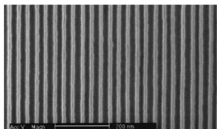
**Fig. 5** SEM of Si nanowire (15 nm wide and 34 nm pitch) mold used for nanoimprinting. Reprinted with permission from ref. 31 (*Nano Lett.*, 2006, **6**, 351–354). Copyright 2006 American Chemical Society.
