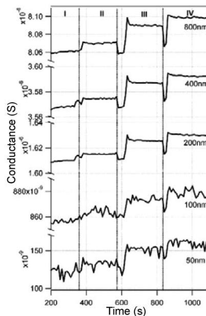
**Fig. 9** Time response of DNA hybridization on five sensors with different dimensions at 4 stages of the experiment. I: DI water; II: 10 nM non-complementary DNA solution; III: 10 pM complementary DNA solution; IV: 100 pM complementary DNA solution. Reproduced from ref. 17 (Li *et al.*, *Appl. Phys. A: Mater. Sci. Process.*, 2005, **80**, 1257–1263) with kind permission of Springer Science and Business Media.
