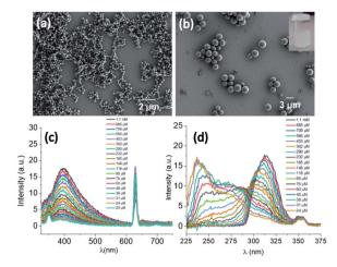
Fig. 2 SEM images of the DPA derivative (a) immediately after preparation and (b) after 24 h of aging. (c) Emission spectra recorded for DPA (1.1 mM) solution on serial dilution in ACN/EtOH/H<sub>2</sub>O (10/40/50%) solvent for  $\lambda_{\rm ex}$  of 315 nm. The peak at 630 nm is the overtone band. (d) Excitation spectra recorded for DPA (1.1 mM) solution for  $\lambda_{\rm em}$  of 397 nm on serial dilution in ACN/EtOH/H<sub>2</sub>O (10/40/50%) solvent.
