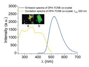
Fig. 8 Emission spectrum for  $\lambda_{\rm ex}$  of 350 nm and excitation spectrum for  $\lambda_{\rm em}$  of 520 nm for the DPA-TCNB co-crystal; inset pictures: (a) optical and (b) confocal microscopy images of the DPA-TCNB co-crystal.
