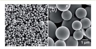
Fig. 12 (a and b) SEM images of pyronin Y doped DPA-TCNB microspheres.
