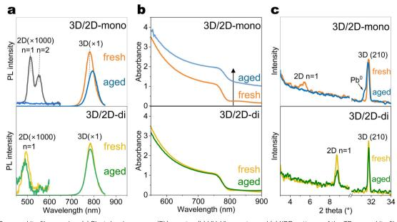
Fig. 2 3D/2D perovskite films ageing. (a) Photoluminescence (PL) spectra, (b) UV-Vis spectra and (c) XRD patterns of the 3D perovskite films coated with mono-ammonium (PEAI) or di-ammonium (BDAI<sub>2</sub>) passivators before and after ageing under light-heat (85 °C and 1-sun illumination) for 300 hours. PEAI and BDAI<sub>2</sub> passivators are respectively labelled as "3D/2D-mono" and "3D/2D-di".
