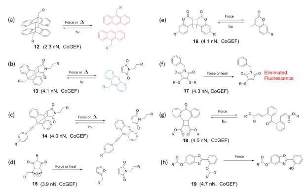
Fig. 5 Structure of various fluorescent mechanophores that are activated by force and display covalent bond scission. (a) Anthracene dimer; (b) Anthracene-maleimide adduct; (c) π-Extended anthracene-maleimide adduct; (d) Furan-maleimide adduct; (e) π-Extended anthracene-maleimide; (g) Methanone-tethered cinnamate dimer. (h) 2-(2'-Hydroxyphenyl)benzoxazole
