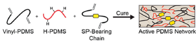
Fig. 22 Schematic representation of SP-containing PDMS network: synthesis route. 44 Fig. 22 is reprinted with permission from ref. 44, Copyright 2014 American Chemical Society.
