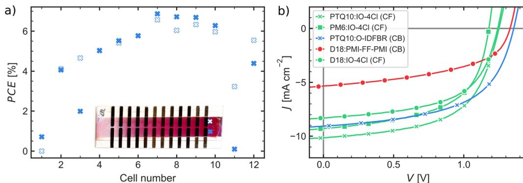
Fig. 2 Thickness dependent efficiency. (a) Power conversion efficiency (PCE) as a function of the cell pixel number (*i.e.* thickness) for a PTQ10:O-IDFBR cell deposited from chloroform solution. The inset shows the substrate with a thickness gradient achieved by varying blade-coater speed. (b)  $J$ - $V$  curves of the best performing cells for each of the six materials tested (donors and acceptors).
