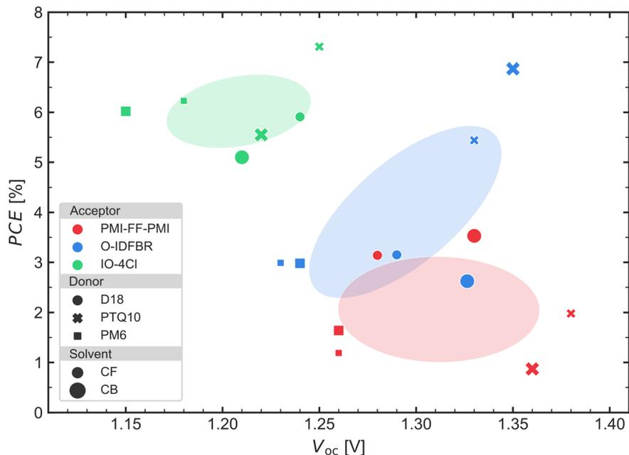
Fig. 3 PCE results. Best power conversion efficiency (PCE) values as a function of the corresponding  $V_{oc}$  achieved for each donor–acceptor–solvent combination. The 18 points are taken from a total of 432 devices where the thickness is optimized for each combination due to the thickness gradient. The coloured ellipses represent confidence regions for the cells containing each acceptor with a  $1\sigma$  confidence.
