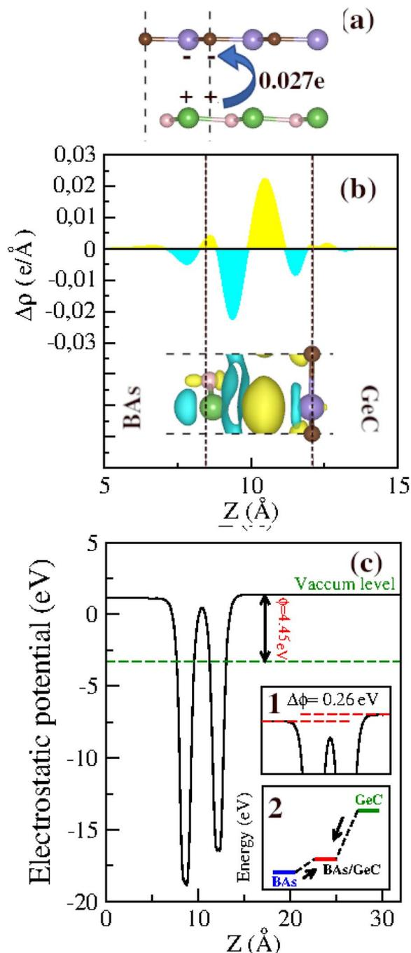
Fig. 6 (a) Bader charge, (b) plane-averaged charge density difference and (c) electrostatic potential of the BAS/GeC heterostructure along the  $z$ -direction. The inset in (b) is the 3D isosurface of the charge density difference.
