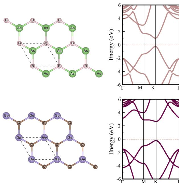
Fig. 2 The left panel illustrates the crystal structures of the isolated BAs and GeC monolayers, and the right panel presents their electronic band structures.
