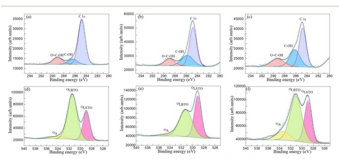
Fig. 4 C 1s spectra of the (a) BST1, (b) BST3 and (c) BST5 photocatalysts. O 1s spectra of the (d) BST1, (e) BST3 and (f) BST5 photocatalysts.
