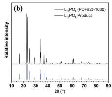
Fig. 3 The  $\text{Li}_3\text{PO}_4$  product precipitated from the 5th enrichment solution. (a) A photographic image of the collected powder. (b) The XRD pattern of the collected powder. All diffraction peaks of the product matched with the standard  $\text{Li}_3\text{PO}_4$  XRD pattern.
