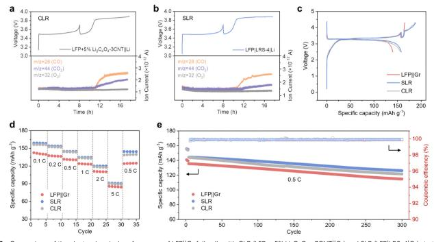
Fig. 3 Comparison of the electrochemical performance of LFP||Gr full cells with CLR (LFP + 5% Li<sub>2</sub>C<sub>4</sub>O<sub>4</sub>-3CNT||Gr) and SLR (LFP|LRS-4|Gr) strategies. (a) and (b) In situ DEMS tests of the LFP||Li half cells. (c) Initial charge-discharge profiles of LFP||Gr full cells. (d) Rate performance of LFP||Gr full cells. (e) Comparison of the cycling stability of the full cells at 0.5C.
