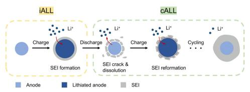
Fig. 1 Schematic of the iALL and cALL that occurs during battery cycling
