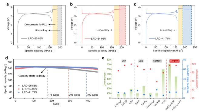
Fig. 6 Anode-supported long-term lithium replenishment strategy (a)-(c) Initial charge-discharge profiles of LFP||Gr full cells with different LRD. (d) Cycling performance of LFP||Gr full cells at 0.5C with additional Li inventory stored in the anode. (e) Comparison of the full cells electrochemical performance with various prelithiation methods. 15,18,21,22,25,38,39
