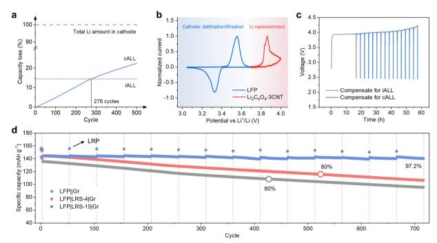
Fig. 5 Electrochemical evaluation of the long-term lithium replenishment strategy (a) the ratio of iALL and cALL after different cycles. (b) CV curves of LFP and  $\text{Li}_2\text{C}_4\text{O}_4$ -3CNT. (c) The controlled-release process verified by LRS-15||Li half cell. (d) Cycling performance of LFP||Gr full cells at 0.5C with longterm lithium replenishment strategy
