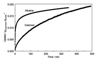
Fig. 24 Neopentane uptake curves for calcined and alkaline-treated ZSM-5 (desilicated) crystals measured using the TEOM (Tapered Element Oscillating Microbalance) at 393 K. The TEOM is a high-precision device that measures real-time changes in mass by detecting variations in the oscillation frequency of a tapered element when molecules are adsorbed or desorbed from the sample. Reproduced with permission from ref. 244. Copyright 2007 American Chemical Society.
