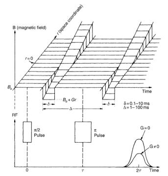
Fig. 6 Sequence of the gradient pulses in PFG NMR. Reproduced with permission from ref. 55. Copyright 2007 Elsevier
