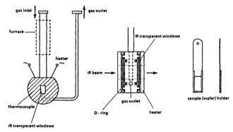
Fig. 15 Experimental setup for measuring diffusivity using FTIR. Reproduced with permission from ref. 90. Copyright 1991 Elsevier.
