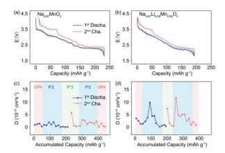
Fig. 5 GITT profiles of (a)  $P'2-Na_{0.67}MnO_2$  and (b)  $P'2-Na_{0.67}Li_{0.05}-Mn_{0.95}O_2$  in a charge and discharge cycle.  $Na^+$  diffusion coefficients of (c)  $P'2-Na_{0.67}MnO_2$  and (d)  $P'2-Na_{0.67}Li_{0.05}Mn_{0.95}O_2$  calculated from GITT measurements.
