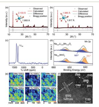
Fig. 1 Rietveld refinement of powder XRD patterns for (a) P'2-Na $_{0.67}$ MnO $_2$  and (b) P'2-Na $_{0.67}$ Li $_{0.05}$ Mn $_{0.95}$ O $_2$ . (c)  $^7$ Li ss-NMR of P'2-Na $_{0.67}$ Li $_{0.05}$ Mn $_{0.95}$ O $_2$ . (d) XPS spectra of the Mn 2p region of Na $_{0.67}$ MnO $_2$  and P'2-Na $_{0.67}$ Li $_{0.05}$ Mn $_{0.95}$ O $_2$ . (e) Elemental SIMS mappings and (f) HRTEM and SAED images of P'2-Na $_{0.67}$ Li $_{0.05}$ Mn $_{0.95}$ O $_2$ .
