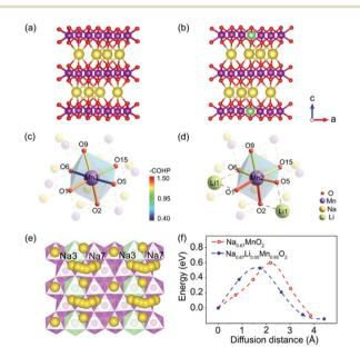
Fig. 4 Optimized structure of (a) P'2-Na $_{0.67}$ MnO $_2$  and (b) P'2-Na $_{0.67}$ Li $_{0.05}$ Mn $_{0.95}$ O $_2$ . COHP analysis of the transition metal octahedral sites of (c) P'2-Na $_{0.67}$ MnO $_2$  and (d) P'2-Na $_{0.67}$ Li $_{0.05}$ Mn $_{0.95}$ O $_2$ . (e) Na3-Na7 diffusion pathway in P'2-Na $_{0.67}$ Li $_{0.05}$ Mn $_{0.95}$ O $_2$ . (f) activation energy barrier for Na $^+$  diffusion in P'2-Na $_{0.67}$ MnO $_2$  and P'2-Na $_{0.67}$ Li $_{0.05}$ Mn $_{0.95}$ O $_2$ .
