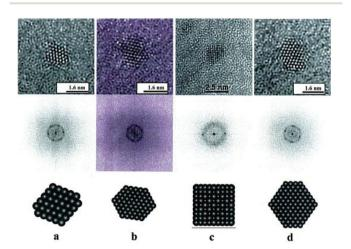
Fig. 11 HREM images of Pd particles with fcc structure. (a) and (b) are in a  $\langle 1\,1\,0\rangle$  orientation and (c) is in a  $\langle 1\,0\,0\rangle$  orientation, while (d) corresponds to a particle with a hexagonal profile, which corresponds to a distorted  $\langle 1\,1\,0\rangle$  orientation. The corresponding FFT is included in each case. Reprinted with permission from ref. 393. Copyright 2001 Elsevier.
