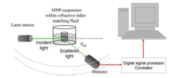
Fig. 2 Optical configuration of the typical experimental setup for dynamic light measurements of a nanoparticle suspension. The setup can be operated at multiple angles. Reproduced with permission from ref. 166. Copyright 2013 Springer.
