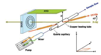
Fig. 1 Schematic presentation of the *in situ* setup employed for realtime SAXS/WAXS/UV-Vis measurements during the formation of Au NPs. The setup measures SAXS, WAXS and the UV-Vis spectra simultaneously in the same sample volume. Reprinted with permission from ref. 43. Copyright 2015 American Chemical Society.
