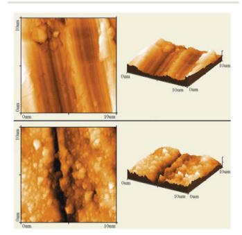
Fig. 22 AFM images of a nickel plate before (upper) and after (lower) the deposition of silver colloidal NPs. Reproduced with permission from ref. 531. Copyright 2007 Elsevier.
