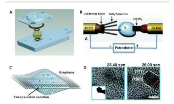
Fig. 13 (A) O-ring sealed *in situ* wet cell design. (B) Sealless *in situ* liquid TEM setup utilizing low vapor ionic liquids. (C) Illustration of an *in situ* liquid cell formed by atomic thin graphene membranes. (D) Atomic resolution images obtained with C, showing the Pt nanocrystal growth procedure. Reprinted with permission from ref. 405. Copyright 2015 Royal Society of Chemistry.
