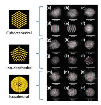
Fig. 15 Typical HAADF-STEM images of thiolated  $(Au_xAg_{1-x})_{312\pm55}$  clusters. (a)–(c), (g)–(i) and (m)–(o) are clusters assigned to cubooctahedral, ino-decahedral or icosahedral structures, based on (d)–(f), (j)–(l) and (p)–(r), the corresponding simulated images (for bare  $Au_{309}$  clusters, which is the closest full shell size of cuboctahedral, icosahedral and inodecahedral). Reprinted with permission from ref. 469. Copyright 2015 American Chemical Society.
