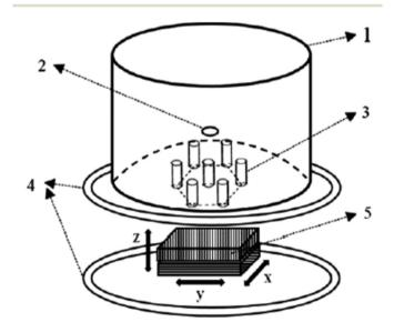
Fig. 8 MRX experimental setup. (1) LiHe Dewar; (2) optional superconducting quantum interference detector (SQUID) magnetometer channel (SQUID sensor not shown); (3) seven-channel second-order SQUID gradiometers (SQUID sensors not shown): (4) Helmholtz coil: and (5) manually controlled non-magnetic 3D stage with optical readout. Reprinted with permission from ref. 352. Copyright 2015 DeGruyter.
