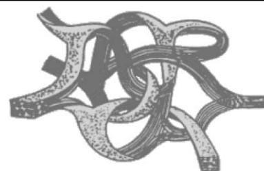
**Glassy carbon** (shown) is comprised of a structure of interwoven ribbons of the graphite structure. This structure means glassy carbon is a much harder form of graphite, and it is impermeable to liquids or gases.
