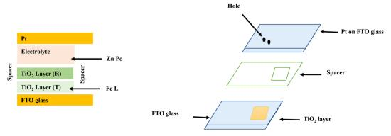
(Left) Structure of a DSSC (Right) photograph of the DSSC package.
