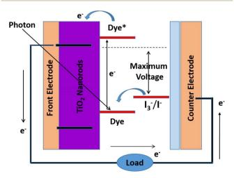
Fig. 4 Sensitize solar cell schematic band diagram.
