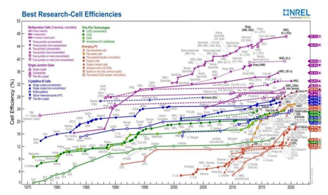
Fig. 2 Year-by-year status of the efficiencies of different PV technologies. Reproduced with permission from National Renewable Energy Laboratory, Golden, CO.
