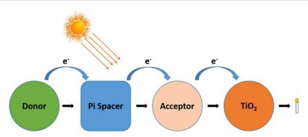
Fig. 6 D- $\pi$ -A (donor-pi-acceptor) dye structure and its functioning in DSSCs.
