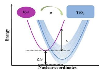
Fig. 7 Energetics of the electron transfer process between a donor (left side) and a quasi-continuum of acceptor states (right side) typical of dye sensitization of a semiconductor.<sup>62</sup>
