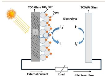
Fig. 3 Layout and functioning of the DSSC diagram.
