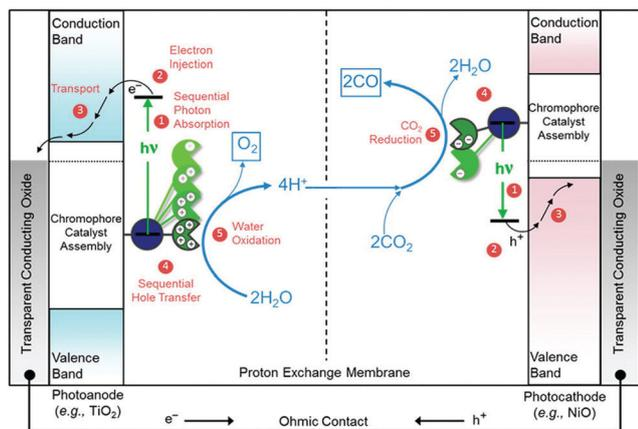
Fig. 52 Schematic diagram for a DSPEC for light-driven  $\text{CO}_2$  splitting into  $\text{CO}$  and  $\text{O}_2$  with an assembly-derivatized  $\text{TiO}_2$  photoanode for water oxidation to  $\text{O}_2$  and an assembly-derivatized photocathode for  $\text{CO}_2$  reduction to  $\text{CO}$ . Reprinted with permission from ref. 735. Copyright 2015 American Chemical Society.
