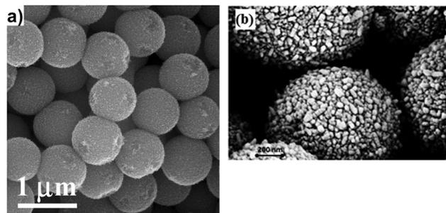
Fig. 17 SEM micrographs of mesoporous  $\text{TiO}_2$  microbeads. (a) Adapted with permission from ref. 223. Copyright 2010 American Chemical Society. (b) Adapted from ref. 222 with permission from The Royal Society of Chemistry, copyright 2014.
