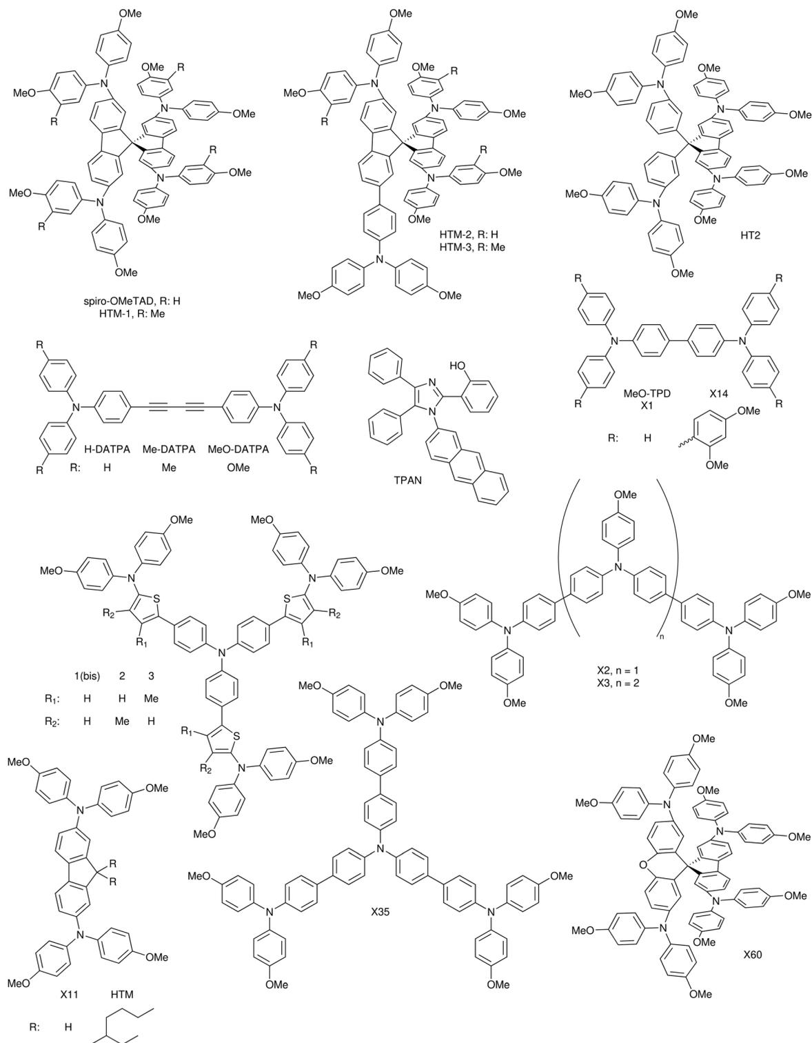
Fig. 37 Examples of triphenylamine-based organic hole conductors.
