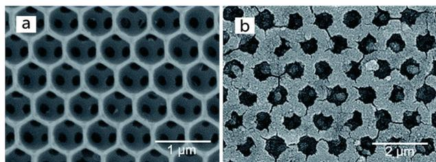
**Fig. 18** (a) Inverse opal SnO<sub>2</sub> electrode; (b) after coating with a 170 nm shell of TiO<sub>2</sub>. Adapted from ref. 235 with permission from The Royal Society of Chemistry, copyright 2016.
