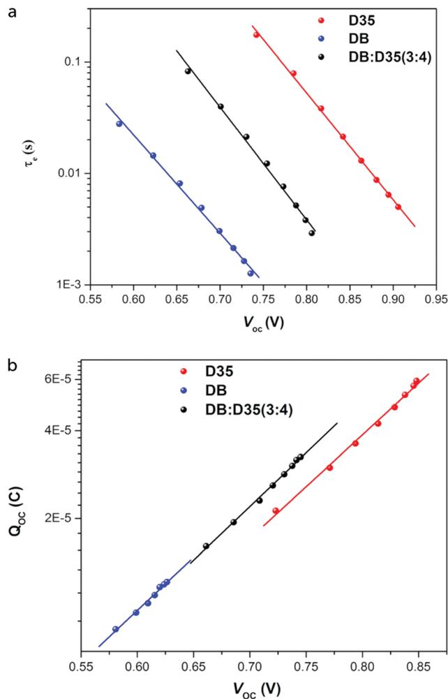
Fig. 9 (a) Electron lifetime and (b) accumulated charge as a function of  $V_{OC}$  for DSCs with a cobalt-based electrolyte, sensitized with D35, Dye-nano blue (DB), or both. Band-edge shifts of the different dyes are small, however a large difference in electron lifetime is found. Adapted with permission from ref. 60. Copyright 2016 American Chemical Society.
