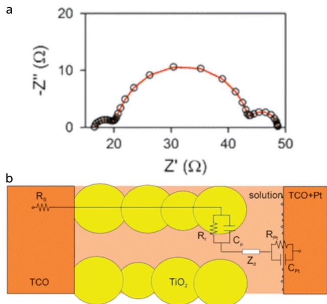
Fig. 7 (a) Impedance spectrum (Nyquist plot) of a dye-sensitized solar cell under illumination, recorded at  $V_{OC}$ . (b) Schematic model to fit the EIS under these conditions. Adapted from ref. 54 with permission from the PCCP Owner Societies, copyright 2011.
