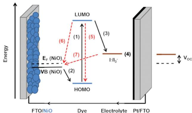
Fig. 42 Schematic representation of the charge transfer processes occurring within a NiO-based p-DSC. Recombination processes shown in red. Processes 1–6 defined in the text. Adapted from ref. 544 with permission from The Royal Society of Chemistry, copyright 2019.
