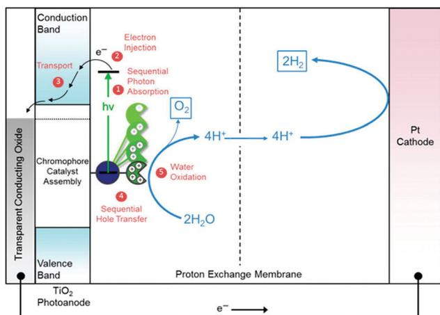
Fig. 48 Schematic diagram of a DSPEC for light-driven water splitting with an assembly-derived TiO<sub>2</sub> photoanode for water oxidation to O<sub>2</sub> and a dark Pt cathode for proton/water reduction to H<sub>2</sub>. Reprinted with permission from ref. 735. Copyright 2015 American Chemical Society.
