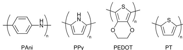
Fig. 41 Repeating units of polymers used as counter electrode materials in DSCs.
