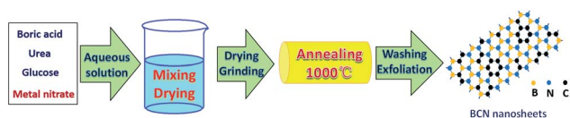
Scheme 1 Schematic diagram for the preparation of BCN nanosheets at low annealing temperature by adding alkaline earth metal compound.
