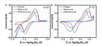
Fig. 2 CV (20 mV s<sup>-1</sup>) thermal re-activation effect on the real and artificially aged felts: (a) negative side and (b) positive side. Measured at a scan rate of 20 mV s $^{-1}$  in an electrolyte of 15 mM VOSO<sub>4</sub>.  $xH_2O$  dissolved in 2 M H<sub>2</sub>SO<sub>4</sub>.
