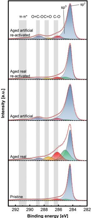
**Fig. 6** Deconvoluted high-resolution XPS spectra of C 1s aged and reactivated anode (positive) felts, compared to pristine thermally activated felt, recorded at pass energy of 27 eV and step size of 0.05 eV.
