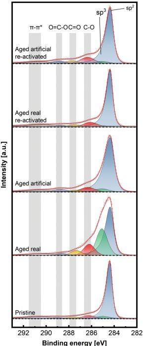
Fig. 7 Deconvoluted high-resolution XPS spectra of C 1s of aged and reactivated cathode (negative) felts, compared to pristine thermally activated felt, recorded at a pass energy of 27 eV and step size of 0.05 eV.
