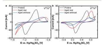
Fig. 1 CV (20 mV s $^{-1}$ ) real and artificial aging: (a) negative side and (b) positive side. Measured at a scan rate of 20 mV s $^{-1}$  in an electrolyte of 15 mM VOSO<sub>4</sub>. xH<sub>2</sub>O dissolved in 2 M H<sub>2</sub>SO<sub>4</sub>.
