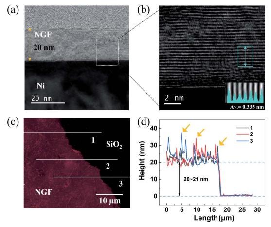
Fig. 6 NGF thickness analysis and cross-sectional TEM images of the NGF: (a) low magnification and (b) higher magnification TEM images of the NGF marked with a white rectangle in (a) and the line-scanning intensity profile (inset bottom-right) obtained from the area highlighted with a cyan rectangle. (c) AFM image of the NGF on the SiO<sub>2</sub>/Si wafer. (d) Thickness profile corresponding to the line shown in (c).
