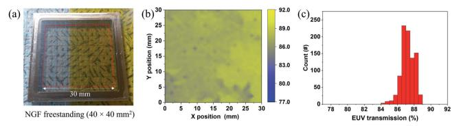
Fig. 5 Measurement of EUV transmittance of the NGF. (a) Photograph of a freestanding NGF ( $40 \times 40 \text{ mm}^2$ ). (b) EUV transmittance mapping image of a NGF with an area of  $30 \times 30 \text{ mm}^2$  marked by a red square in (a). (c) Histogram of EUV transmission.
