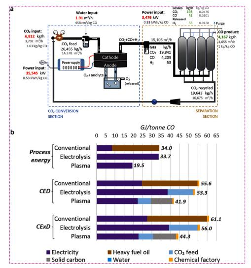
Fig. 41 (a) Schematic flow diagram illustrating the operation of an electrolyser-based facility designed to produce 100 tonnes of carbon monoxide. (b) Comparison of energy costs associated with conventional, electrolysis-based, and plasma-based CO production methods, based on their respective baseline scenarios. Reproduced from ref. 350 with permission from Royal Society of Chemistry (CC-BY 4.0), copyright 2024
