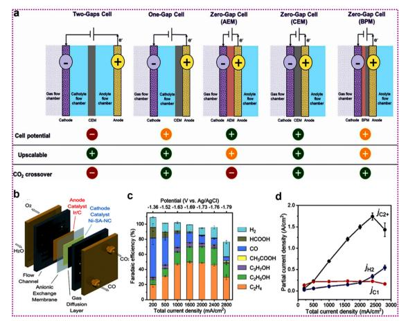
Fig. 40 (a) Configuration of various electrochemical cells (AEM, PEM, BPM). Reproduced from ref. 346 with permission from Elsevier (CC-BY 4.0), copyright 2024. (b) Typical membrane electrode assembly. (c) FEs under various applied potentials catalyzed by CuONPs in 1 M KCl. (d) Partial current density of eCO<sub>2</sub> reduction products catalyzed by CuONPs in 1 M KCl. Reproduced from ref. 347 with permission from Royal Society of Chemistry (CC-BY 4.0), copyright 2023.
