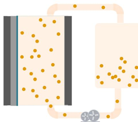
Fig. 8 Schematic illustration of liquid/solid membrane-free RFB.
