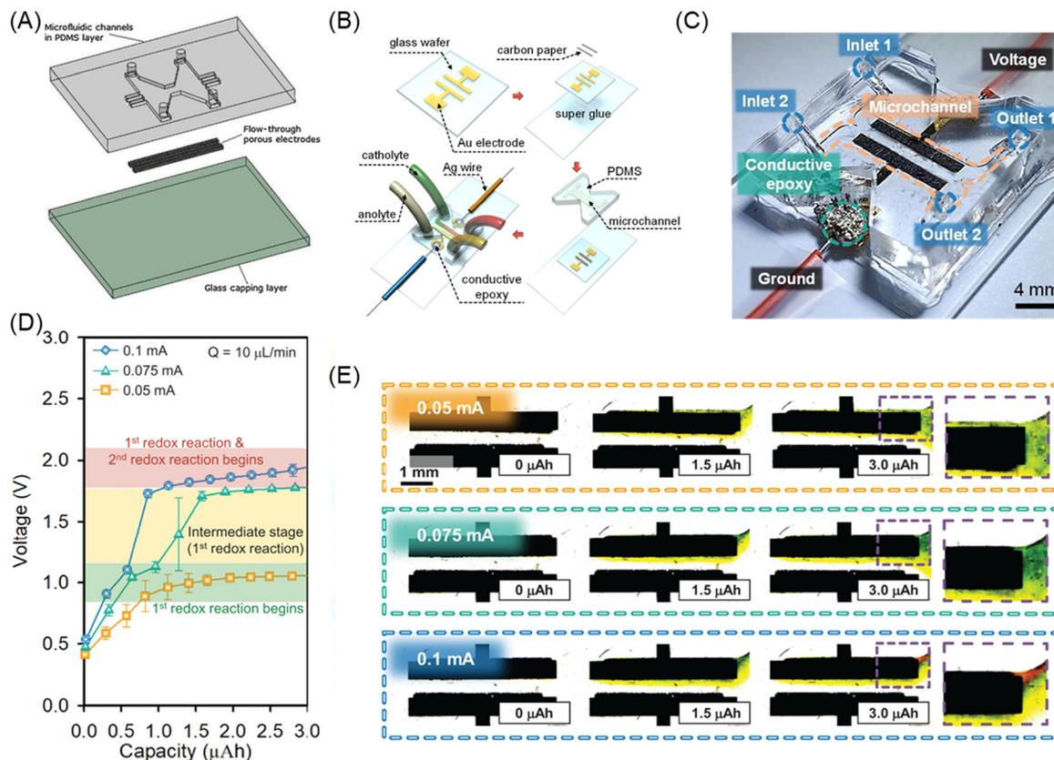
Fig. 7 (A) Typical single-phase co-laminar flow battery. (B) Microscale fabrication process and (C) digital photograph of the microfluidic membrane-free RFB. (D) Voltage and capacity profiles of the membrane-free RFB using the redox couple in terms of charge transfer and (E) in *operando* visualization of the electrochemical reaction. Reproduced from ref. 43 with permission from the National Academy of Sciences, copyright 2022.
