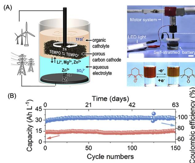
Fig. 3 (A) Schematic illustration and digital photographs of stirred self-stratified battery. (B) Cycling performance of a  $20 \text{ W h L}^{-1}$  stirred self-stratified battery. Reproduced with permission from ref. 29. Copyright 2020, Elsevier.
