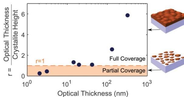
**Fig. 3** Ratio of the thickness determined from the absorption coefficient (optical thickness), and the grain height calculated from XRD FWHM. When the ratio is equal to one or more, the surface of the substrate is fully covered, as illustrated.
