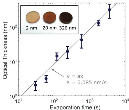
**Fig. 1** Thickness calculated by matching the absorbance of each sample to a known absorption coefficient in the range 550–700 nm (optical thickness). The grey line is the fit ( $y = ax$ ) to the data, giving a deposition rate of  $0.085 \text{ nm s}^{-1}$ . The inset is a photograph of the 2, 20 and 320 nm MAPbI<sub>3</sub> films on 2 mm-thick quartz substrates, showing that the difference in absorption can be seen by eye.
