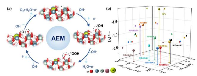
Fig. 1 (a) AEM on NiFeMnM(oxy)hydroxide. (b) Three-dimensional reaction energy barrier model.
