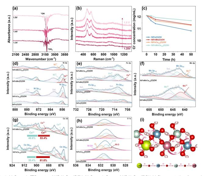
Fig. 4 (a) Operando FTIR spectra of NiFeMnCe<sub>0.8</sub>(O)OH. (b) Operando Raman of NiFeMnCe<sub>0.8</sub>(O)OH. (c)  $Cl^-$  concentration after reaction determined by IC. XPS spectra of (d) Ni 2p, (e) Fe 2p, (f) Mn 2p, (g) Ce 3d and (h) O 1s. (i) Schematic diagram of charge transfer.
