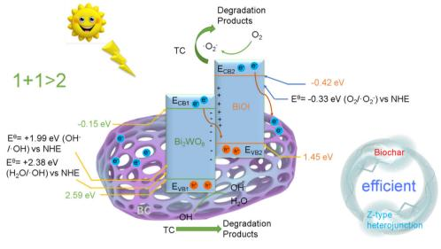
Fig. 10 Possible path and photocatalytic mechanism of photocatalytic TC degradation by BC/BWI under solar radiation.
