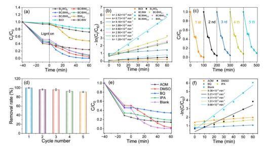
Fig. 7 (a) Adsorption and degradation curves of TC; (b) kinetics of TC degradation; (c) and (d) reusability of Bi<sub>2</sub>WO<sub>6</sub> in five runs for TC. (e) and (f) scavenger experiments and kinetic fitting ( $t_0$  represents the concentration of TC at the time of illumination).
