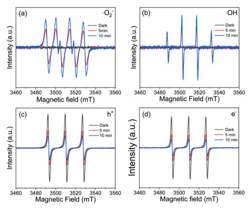
Fig. 8 ESR spectrum of (a) DMPO-'O<sub>2</sub>-'; (b) DMPO-'OH; (c) TEMPO-h<sup>+</sup> and (d) TEMPO-e<sup>-</sup> under both the dark and visible light irradiation.
