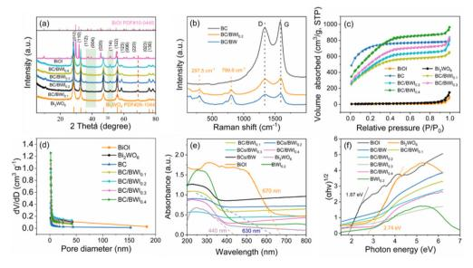
Fig. 3 (a) XRD patterns of Bi<sub>2</sub>WO<sub>6</sub>, BC/BWI<sub>0.1</sub>, BC/BWI<sub>0.2</sub>, BC/BWI<sub>0.3</sub>, BC/BWI<sub>0.4</sub>, and BiOI. (b) Raman shift pattern of BC, BC/BW and BC/BWI<sub>0.2</sub>; (c) the N<sub>2</sub> adsorption-desorption isotherms and (d) pore size distribution of samples; (e) UV-vis diffuse reflectance spectra and (f) plot of Kubelka-Munk transformation of samples.
