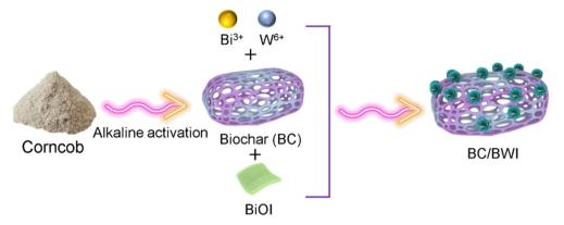
Fig. 1 Synthesis process of BC/BWI.
