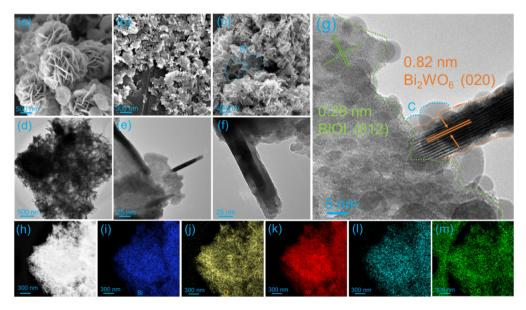
Fig. 2 SEM images of (a) Bi<sub>2</sub>WO<sub>6</sub>, (b) BiOI, and (c) BC/BWI<sub>0.2</sub>; (d-g) TEM and HR-TEM images of BC/BWI<sub>0.2</sub>; elemental mapping images (h) and (i-m) the element distribution of C, O, W, Bi and I of BC/BWI<sub>0.2</sub>.
