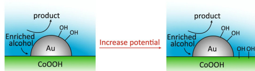
Fig. 8 (a) Traditional electrochemical oxidation of alcohol process over Au catalyst and its deactivation at high potential. (b) Alcohols enrichment and reactive adsorbed OH generation over the interface of Au/CoOOH. Adapted with permission from ref. 18. Copyright 2022, The Author(s).
