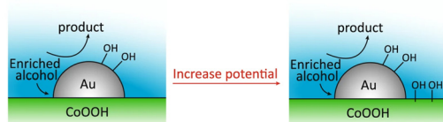
Fig. 8 (a) Traditional electrochemical oxidation of alcohol process over Au catalyst and its deactivation at high potential. (b) Alcohols enrichment and reactive adsorbed OH generation over the interface of Au/CoOOH. Adapted with permission from ref. 18. Copyright 2022, The Author(s).
