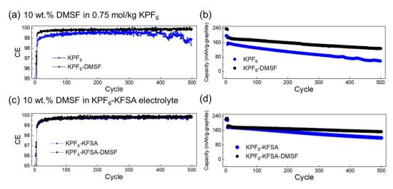
Fig. 5 Extended cycling performance of graphite  $\parallel$  Mn-PB cells with 10 wt% DMSF. (a) CE and (b) extracted discharge capacities for cells cycled in 0.75 mol kg<sup>-1</sup> KPF<sub>6</sub> in EC: DEC with or without 10 wt% DMSF at 1C. (c) CE and (d) extracted discharge capacities for cells cycled in an optimized KFSA-KPF<sub>6</sub> mixed electrolyte<sup>9</sup> with or without 10 wt% DMSF at 1C.
