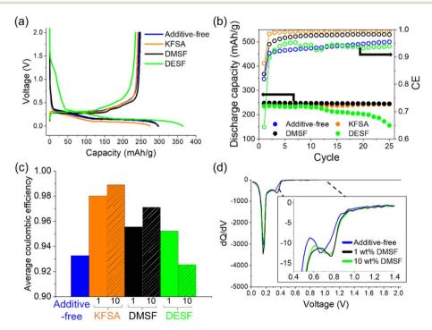
Fig. 2 Half-cell cycling with fluorosulfonamide additives. (a) 1st cycle charge—discharge curves and (b) extracted results after further cycling at 0.1C in a graphite K cell with 10 wt% additives. (c) Comparison of average CEs with 1 and 10 wt% additives. (d) Differential capacity curves of the first charge for cells that were additive-free or contained 1 and 10 wt% DMSF.
