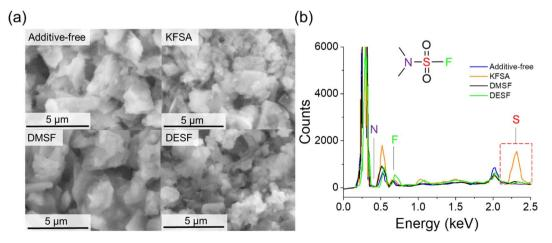
Fig. 6 SEM and EDS measurements on cycled graphite electrodes. (a) SEM images of graphite electrodes after 10 cycles in cells containing 10 wt% of each additive. (b) EDS results of each cell.
