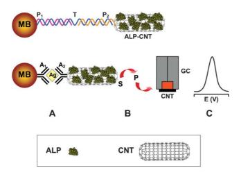
Fig. 5 Ultrasensitive bioassays of proteins and nucleic acids based on the amplification features of carbon-nanotube carriers and modified electrodes. (Based on ref. 44 with permission.)
