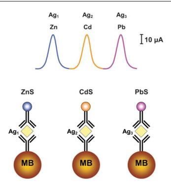
**Fig. 3** Multi-antigen sandwich immunoassay protocol based on different inorganic-colloid (quantum dots) nanocrystal tracers. (Based on ref. 36 with permission.)
