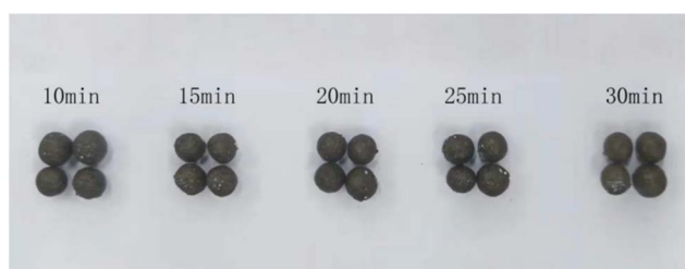
Fig. 15 Morphology of ceramics at different sintering time.
