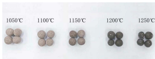
Fig. 12 Morphology of ceramsite at different sintering temperatures.
