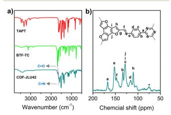
Fig. 2 (a) FT-IR spectra of COF-JLU42 and corresponding monomers. (b) Solid-state <sup>13</sup>C spectra of COF-JLU42, inset: the chemical structure of COF-JLU42. Asterisk (\*) indicates a peak arising from a spinning band.
