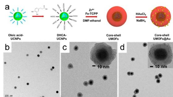
Fig. 13 (a) Illustration depicting the formation of core–shell UMOFs@Au NPs. TEM images of (b) carboxylic acid stabilized UCNPs in aqueous solution, UMOF NPs (c), and UMOF@Au NPs (d). (Panels a–d) Reproduced with permission.<sup>6</sup> Copyright 2020, American Chemical Society.
