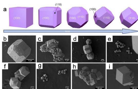
**Fig. 2** (a) Evolution of ZIF-67 crystal morphology over time. SEM micrographs were taken after 15 min (b and c), 20 min (d and e), 45 min (f and g), and 240 min (h and i). Panels (a–i) Reproduced with permission.<sup>4</sup> Copyright 2012, Royal Society of Chemistry.
