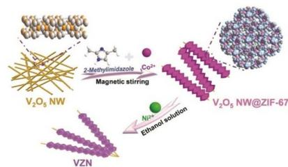
**Fig. 3** Schematic illustration of the preparation of ZIF-67 on  $V_2O_5$  NWs (VZN). (Panels) Reproduced with permission.<sup>1</sup> Copyright 2023, Wiley.
