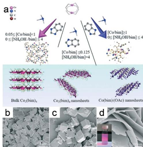
Fig. 8 (a) The diagram depicts the process for the synthesis of the  $\text{Co}_2(\text{bim})_4$ , the  $\text{UTCo}_2(\text{bim})_4$ , as well as the  $\text{Co}(\text{bim})(\text{OAc})$  nanosheets prepared using varying amounts of  $\text{NH}_4\text{OH}$  ( $Y$  value denotes the  $\text{NH}_4\text{OH}/\text{bim}$  molar ratio): (b)  $Y = 0$ ; (c)  $Y = 2$ ; (d)  $Y = 4$ . (Panels a–d) Reproduced with permission.<sup>19</sup> Copyright 2019, Royal Society of Chemistry.
