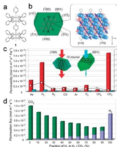
Fig. 17 (a and b) The crystal structure of [Cu<sub>2</sub>(bza)<sub>4</sub>(pyz)]<sub>n</sub> (1) with calculated crystal plane numbers and channel direction. (c) The comparison of gas permeabilities through the crystal membrane 1. (d) Comparative analysis of the flow rates of H<sub>2</sub> and CO<sub>2</sub> passing through the channels of gas mixtures at varying mixing ratios. (Panels a–d) Reproduced with permission.<sup>12</sup> Copyright 2010, American Chemical Society.
