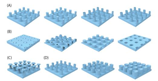
Fig. 14 The development of octopus-inspired wet adhesive structures. (A) Suckers with different curvature radii ( $\sim 1.00$ ,  $\sim 0.66$ ,  $\sim 0.84$ ,  $\sim 0.93$ ). (B) Suckers with different shapes, including octopus-inspired architecture, perforated cylinders, cylindrical pillars and cylindrical holes. (C) Hierarchical micropillars with suckers on top. (D) Suckers with different diameter sizes (15, 50, and 500  $\mu$ m in diameter) with  $\sim$ 0.93 curvature.
