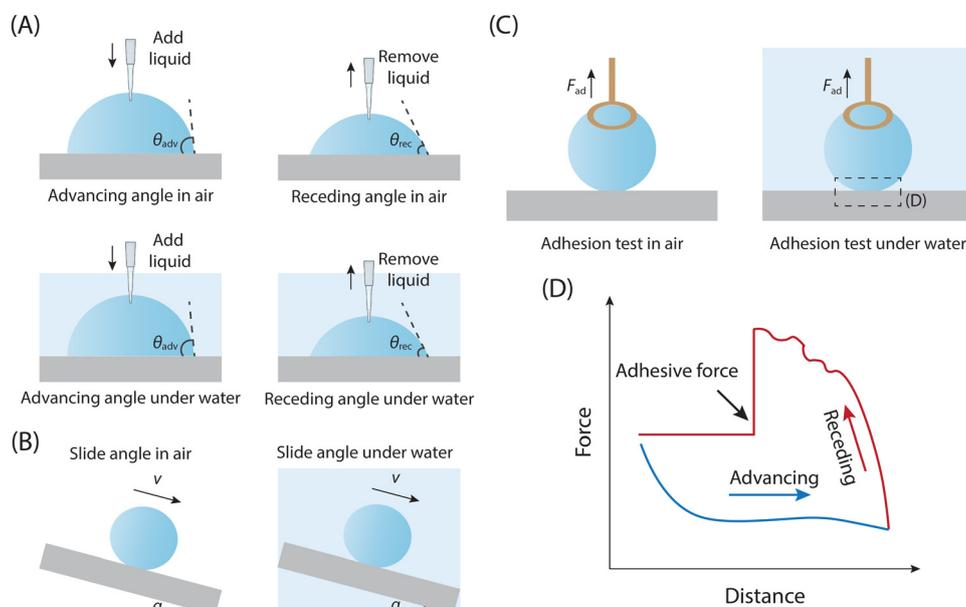
Fig. 4 Illustration of commonly used interfacial adhesion test methods for solid–liquid adhesion (including both in air and underwater environment). (A) Droplet advancing & receding angle ( $\theta_{Adv}$  &  $\theta_{Rec}$ ) test. (B) Droplet sliding angle test. (C) Droplet adhesive force test. (D) Typical force–distance curve for droplet adhesive force test.
