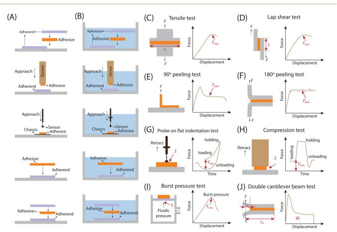
Fig. 5 Illustration of commonly used interfacial adhesion test methods for solid–solid/solid–liquid-solid adhesion(including both in air and underwater environment). (A) and (B) Pretreatments for different adhesion tests, (A) in air, (B) underwater. (C) Tensile test. (D) Lap shear test (E) 90° peeling test (F) 180° peeling test. (G) Probe on flat test. (H) Flat punch test. (I) Burst pressure test. (J) Double cantilever beam (DCB) test.
