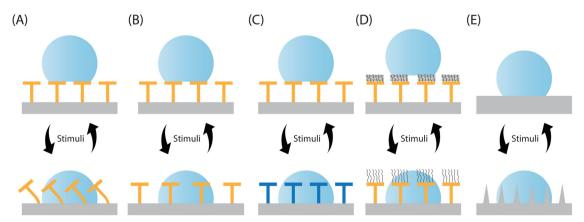
Fig. 18 Construction strategies to control surface wetting and adhesion for solid structure surfaces. (A) Modulating the physical shape of micro-nano structures. (B) Modulating the distribution and morphology of micro-nanostructures on the surface through stretching or bending of the substrate. (C) Modulating the chemical properties of micro-nano structures. (D) Modulating the acting state of functional molecules. (E) Modulating the formation or disappearance of microneedles
