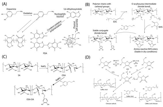
Fig. 10 Schematics of typical modification methods for incorporating catechol and its derivatives into polymers. (A) Self-polymerization of dopamine. (B) 1-Ethyl-3-(3-dimethylaminopropyl) carbodiimide/N-hydroxysuccinimide (EDC/NHS) coupling chemistry. (C) Schiff-base chemistry. (D) The free radical-induced grafting method using the ascorbic acid/H<sub>2</sub>O<sub>2</sub> redox system.
