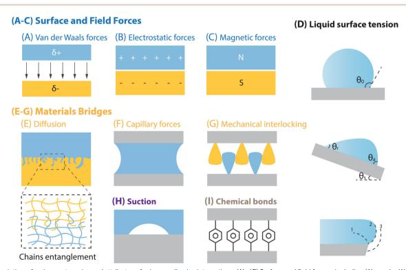
Fig. 2 Depiction of various categories and attributes of primary adhesive interactions. (A)–(C) Surface and field forces, including (A) van der Waals forces, (B) electrostatic forces and (C) magnetic forces. (D) Liquid surface tension, which helps liquids to adhere to solid surfaces in the form of drops. (E)-(G) Material bridging, encompassing (E) diffusion, (F) capillary forces and (G) mechanical interlock. (H) Suction forces. (I) Chemical bonds.
