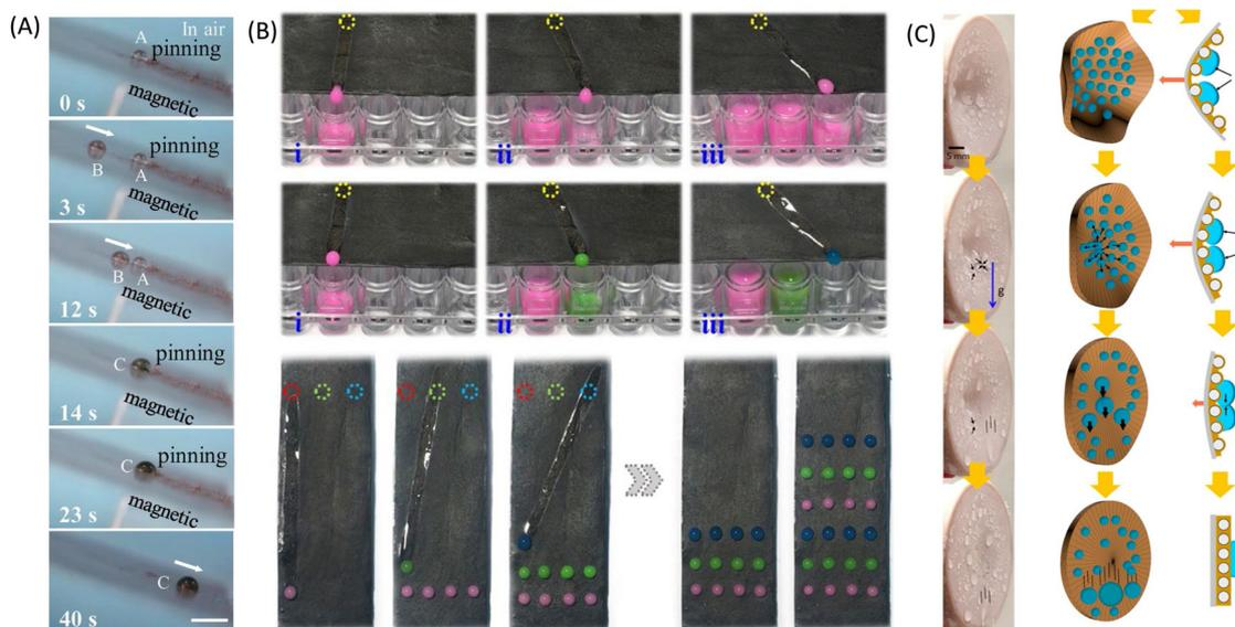
**Fig. 23** Bioinspired adhesives for droplet manipulation. (A) Responsive SLIPs serve as microreactors. The picture is reproduced with permission from ref. 408 Copyright 2019, Wiley-VCH. (B) Responsive SLIPs serve as pipetting devices. The picture is reproduced with permission from ref. 502 Copyright 2018, AAAS. (C) Responsive SLIPs used for collecting water and fog in the air. The picture is reproduced with permission from ref. 444 Copyright 2017, American Chemical Society.
