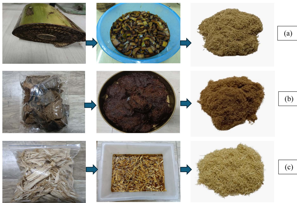
Fig. 1 Extraction of fibres from (a) raw banana pseudo-stem, (b) raw coconut coir, and (c) raw sugarcane bagasse.
