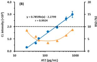
Fig. 4 The calibration curve (ullet) and precision profile (ullet) of the proposed CLEIA for ATZ. The CL intensity values were plotted *versus* concentrations of ATZ on linear (A) and logarithmic (B) scales, respectively.
