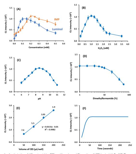
Fig. 3 The results of optimization of different variables CES used for enhanced CL reaction of HRP-luminol- $H_2O_2$ -IMP. These variables are the concentrations of luminol and IMP (A), concentration of  $H_2O_2$  (B), pH (C), concentration of dimethylformamide (D), volume of CES (E), and reaction time (F). The values are mean of 3 measurements  $\pm$  SD.
