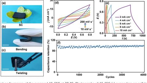
Fig. 3 Electrochemical performance of the prepared AF-FSC at 20 °C. Photographs of AF-FSC (a) supporting on soft leaves; (b) bending; (c) twisting. (d) CV and (e) GCD curves of the AF-FSC at different scan rates or current densities. (f) Cycling performance of the AF-FSC at  $100 \text{ mV s}^{-1}$ .
