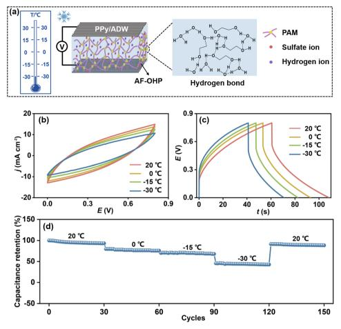
Fig. 4 The anti-freezing property of the SC. (a) Schematic illustration of the SC at -30 °C. Comparison of (b) CV and (c) GCD curves of the SC at temperatures of 20, 0, -15 and -30 °C. (d) Cycling performance of the SC at 20, 0, -15 and -30 °C. Scan rate of CV: 100 mV s<sup>-1</sup>; current density of GCD: 6 mA cm<sup>-2</sup>
