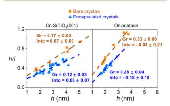
Fig. 15 Aspect ratio of Pd crystals plotted against their height for Pd crystals on nanostructured SrTiO<sub>3</sub> (001) and anatase (001) substrates. Adapted with permission from ref. 102. Copyright 2021, American Physical
