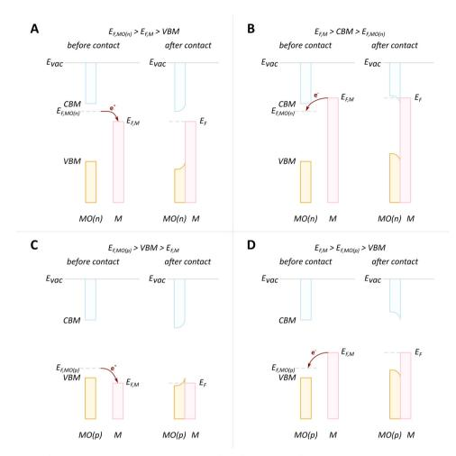
Fig. 7 Schematic diagrams of charge redistribution and band bending for different cases of doping types and Fermi level positions. (A) n-type donordoped MO with Fermi level of MO higher than that of metal; (B) n-type donor-doped MO with Fermi level of MO lower than that of metal; (C) p-doped MO with Fermi level of MO higher than that of metal; (D) p-doped MO with Fermi level of MO lower than that of metal. Adapted with permission from ref. 84. Copyright 2015, Springer Nature.
