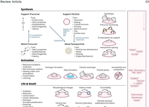
Fig. 17 Schematic overview of the means through which MSI can be tuned, as well as the resulting physicochemical properties affected by these means throughout the lifetime of a catalyst (i.e., during synthesis, activation, reaction, deactivation). The right side of the figure shows typically used abbreviations in literature, and the point in the lifetime of a catalyst when they are at play.
