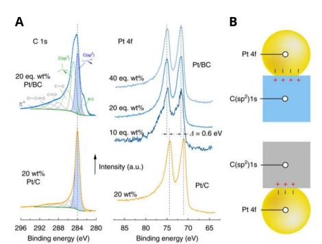
Fig. 20 (A) XPS spectra of the C 1s and Pt 4f region of the Pt/C and Pt/BC catalysts. Spectra are aligned to the graphitic C (sp<sup>2</sup>) peak at 284 eV; (B) schematic of charge transfer across the support/catalyst interface due to Fermi level equilibration rationalizing relative shifts in the XPS Pt 4f and C 1s core levels. Adapted from ref. 222
