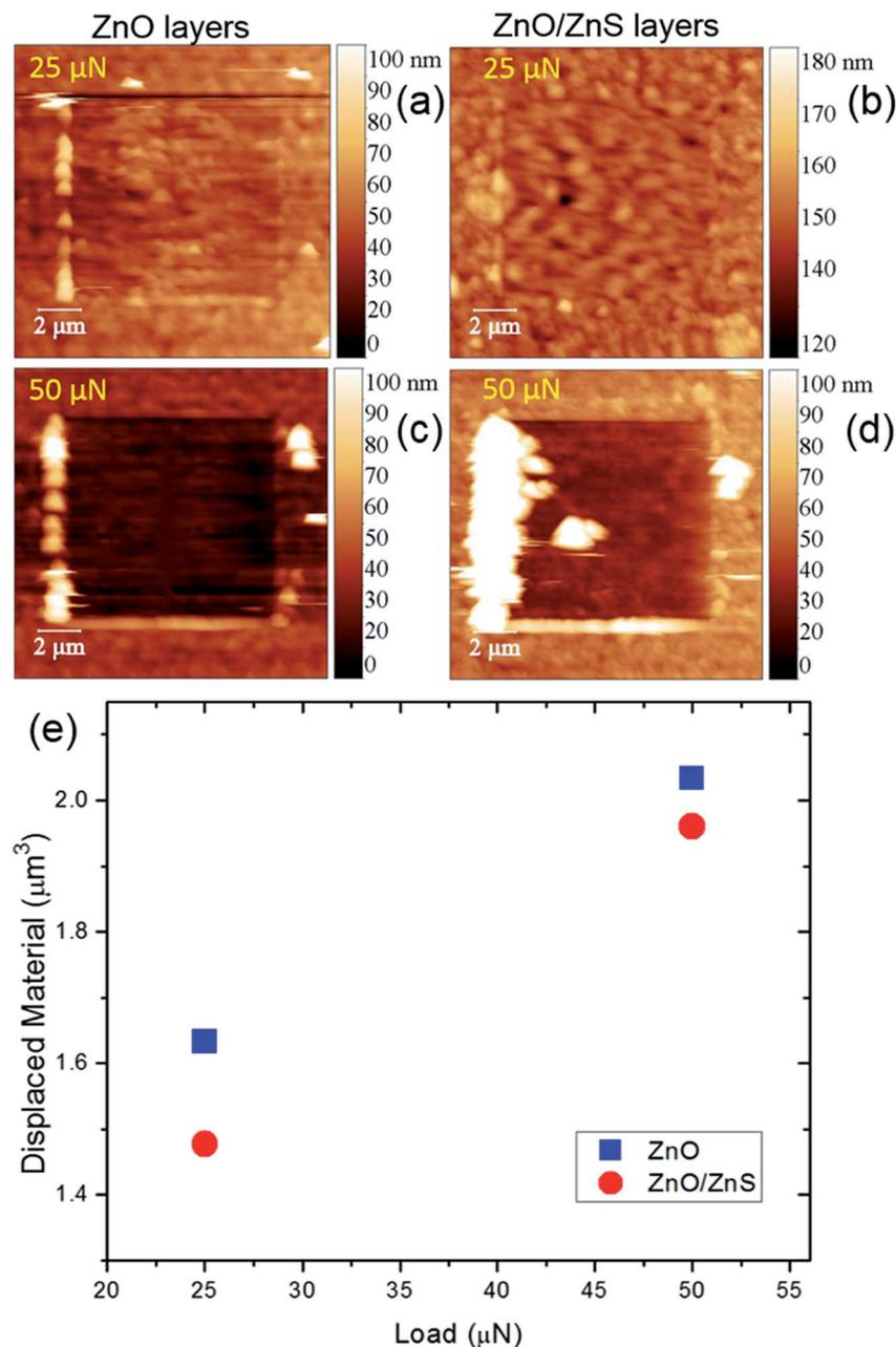
Fig. 6 (a and c) ZnO and (b and d) ZnO/ZnS nanofilms after a nanowear test performed by holding a constant force of (a and b) 25 and (c and d) 50  $\mu\text{N}$  and (e) the values of the displaced material calculated by the residual imprint.
