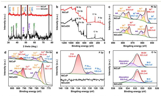
Fig. 2 (a) XRD patterns and XPS spectra of (b) broad scans, (c) Ni 2p, (d) Co 2p, (e) P 2p and (f) O 1s of NiCoP and NiCoOH electrocatalysts.
