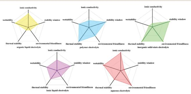
Fig. 1 Semi-quantitative comparison of organic liquid electrolyte, polymer electrolyte, inorganic solid-state electrolyte, ionic liquid electrolyte and aqueous electrolyte.
