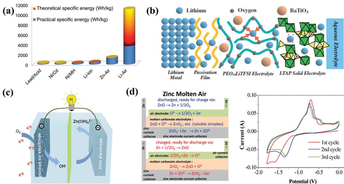
Fig. 4 (a) Theoretical and practical energy densities of various types of rechargeable batteries.<sup>118</sup> (b) Schematic diagram of the proposed water stable lithium metal electrode with polymer buffer layer and glass ceramic separator.<sup>120</sup> (c) Schematic principle of operation for Zn//air batteries.<sup>123</sup> (d) Schematic representation of the molten Zn//air battery and CV curve of Zn redox reaction in that electrolyte with a sweep rate of 100 mV s<sup>-1</sup>.<sup>125</sup>
