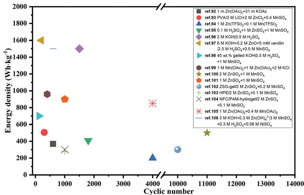
Fig. 3 Performance comparison of recently reported Zn//MnO<sub>2</sub> batteries based on various aqueous electrolytes in terms of energy density and cyclic number.
