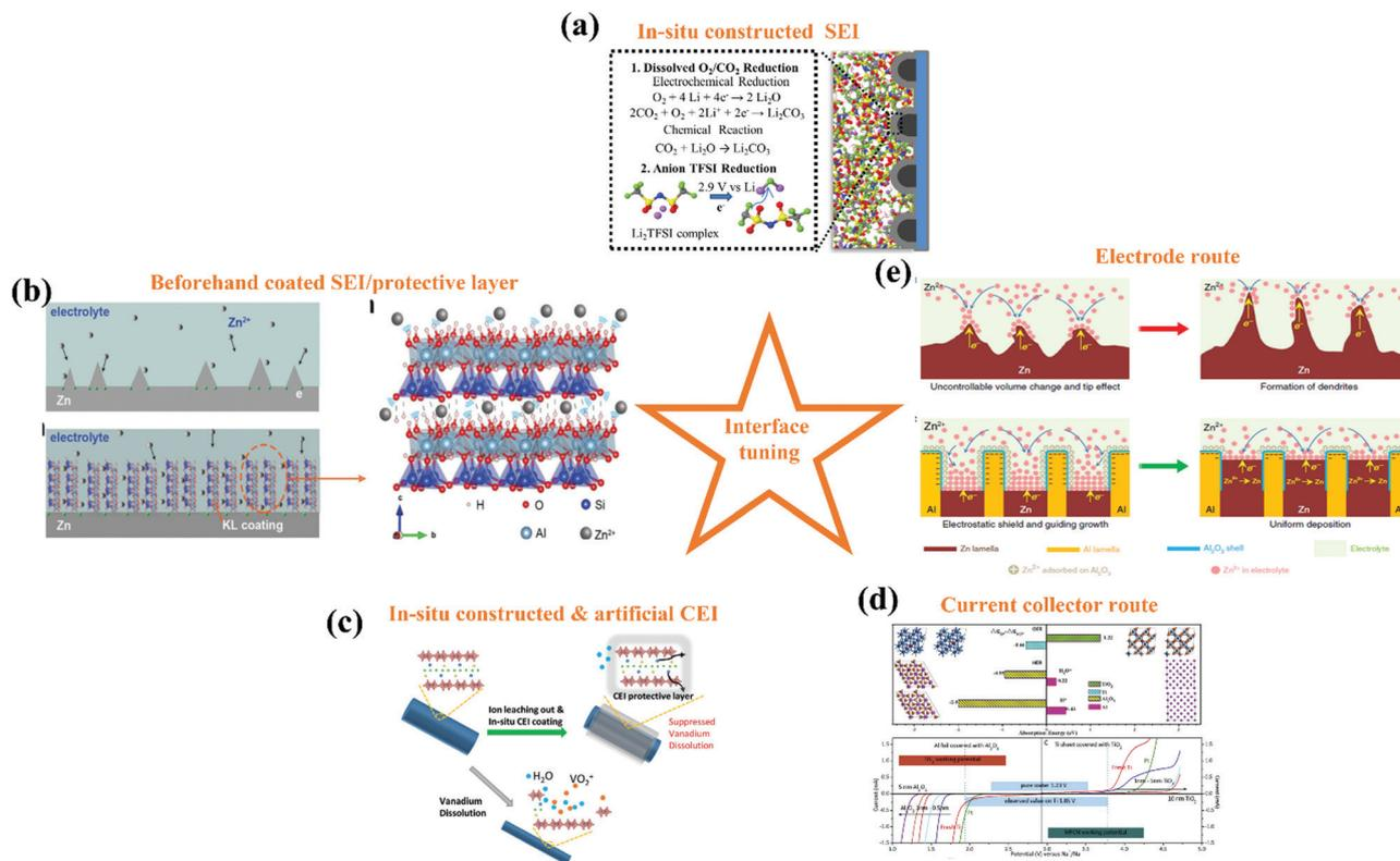
Fig. 14 (a) SEI formation mechanisms in WiSE.<sup>246</sup> (b) Schematic diagrams of Zn deposition process on bare Zn and KL–Zn with a detailed schematic diagram of confined  $Zn^{2+}$  transmission in kaolin.<sup>250</sup> (c) Illustration of the *in situ* CEI layer strategy design.<sup>252</sup> (d) Stability of Al and Ti current collectors in 15 m  $NaClO_4$  aqueous electrolyte.<sup>254</sup> (e) Schematic illustration of eutectic strategy for dendrite and crack suppression.<sup>257</sup>
