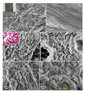
Fig. 1 FESEM images of EG (a and b), EG/Co<sub>0.85</sub>Se (c and d), and EG/ Co<sub>0.85</sub>Se/NiFe-LDH (e and f). Inset: The corresponding EG photograph (a) and the enlarged FESEM image of EG/Co<sub>0.85</sub>Se (c).
