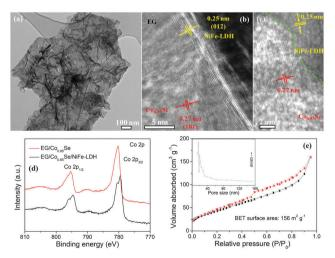
Fig. 2 TEM (a) and HRTEM (b and c) images of EG/Co $_{0.85}$ Se/NiFe-LDH. (d) High-resolution Co 2p XPS spectra of EG/Co $_{0.85}$ Se and EG/Co $_{0.85}$ Se/NiFe-LDH. (e) N $_{2}$  adsorption isotherm and the corresponding pore size distribution (inset) of EG/Co $_{0.85}$ Se/NiFe-LDH.
