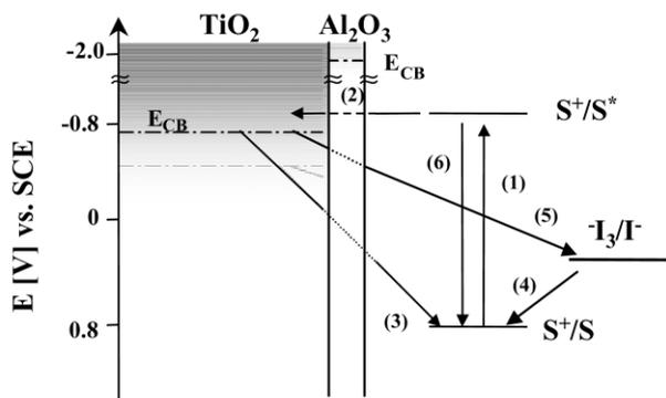
**Scheme 1** Illustration of the interfacial charge-transfer processes occurring at the nanostructured TiO<sub>2</sub>/dye/electrolyte interface of DSSC. Also shown is the Al<sub>2</sub>O<sub>3</sub> blocking layer as developed in this paper.
