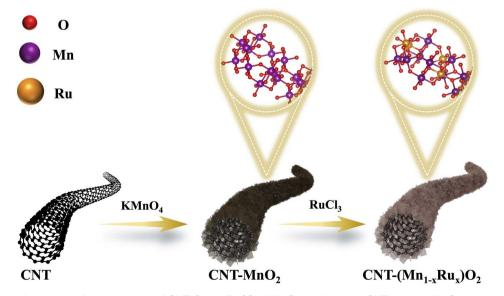
Scheme 1 Schematic illustration of the synthesis of CNT- $(Mn_{1-x}Ru_x)O_2$ . KMnO<sub>4</sub> oxidizes the CNT to form MnO<sub>2</sub>-coated CNT (CNT-MnO<sub>2</sub>), followed by RuCl<sub>3</sub> treatment to generate Ru-substituted (Mn<sub>1-x</sub>Ru<sub>x</sub>)O<sub>2</sub> domains confined on the CNT surface. The inset highlights the atomic-level incorporation of Ru into the MnO<sub>2</sub> lattice, forming CNT-Mn-O-Ru bridges.
