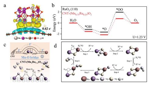
Fig. 5 (a) Charge distribution analysis of CNT- $(Mn_{0.75}Ru_{0.25})O_2$ . Yellow region indicates charge accumulation, while the blue region indicates charge reduction. (b) The calculated reaction pathways of CNT- $(Mn_{0.75}Ru_{0.25})O_2$  and  $RuO_2(110)$  for acidic OER at U=1.23 V. Schematic illustration of the LOM pathway during acidic OER and (c and d) enhanced LOM pathway in CNT- $(Mn_{\chi}Ru_{1-\chi})O_2$  with improved oxygen vacancy dynamics and structural stability.
