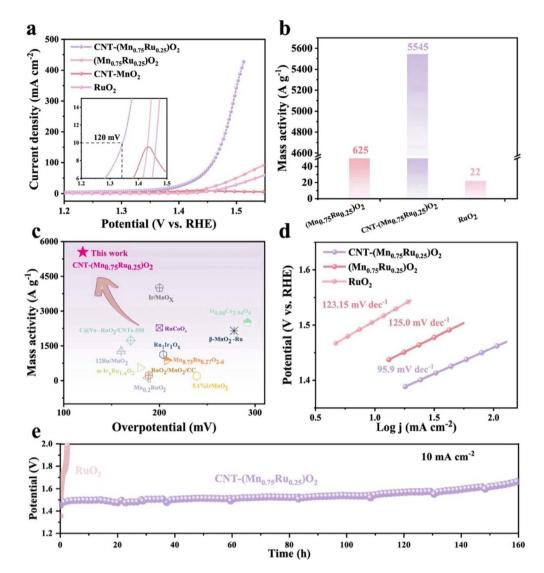
Fig. 3 (a) OER performance of the catalysts in 0.1 M  $HClO_4$  solution. (b) Mass activity at 1.5 V of the catalysts. (c) Comparison of OER overpotential and mass activity of previously reported electrocatalysts. (d) Tafel slope of the catalysts. (e) Durability test of CNT-( $Mn_{0.75}Ru_{0.25}$ )O<sub>2</sub> and  $RuO_2$ .
