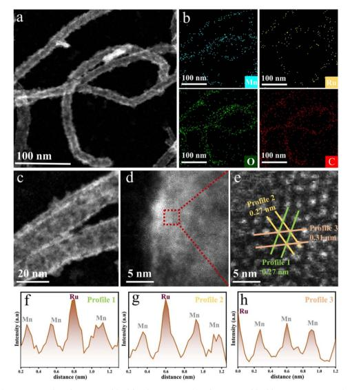
Fig. 1 (a) HAADF-STEM image of CNT- $(Mn_{0.75}Ru_{0.25})O_2$ . (b) EDS mapping of CNT- $(Mn_{0.75}Ru_{0.25})O_2$ . (c) High-magnification STEM image showing the morphology from (a). (d) Atomic-resolution STEM image of a representative part selected from (c). (e) Enlarged view of the red-boxed region in (d). (f–h) The corresponding intensity profile of the line regions in (e).
