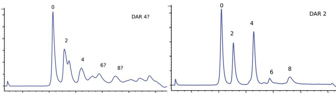
**Fig. 2** HIC-UV/Vis spectrum for an early cysteine-linked ADC construct with DAR of approximately 4 (Left) and a cysteine-linked ADC construct with DAR 2 (Right) with different DAR species assigned to each peak when possible. As can be observed the annotation of DAR to specific peaks is not always straightforward even for cysteine-linked ADCs in HIC-UV/Vis.
