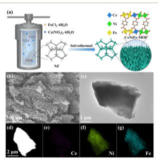
Fig. 1 (a) Schematic synthesis of CeNiFe-MOF on nickel foam. (b) SEM, (c) TEM and (d-g) elemental mapping images of CeNiFe-MOF.
