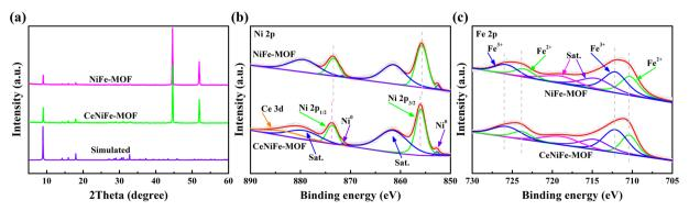
Fig. 2 (a) XRD patterns, (b) Ni 2p and (c) Fe 2p spectra of NiFe-MOF and CeNiFe-MOF.
